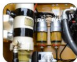
Centralized 3 Stage Fuel Filtration System
