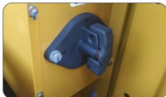
Battery cutoff switch
